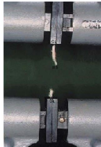
Figure 8.12 A tissue sample being tested for tensile strength using an Instron machine. Picture courtesy of M. Calvin.
