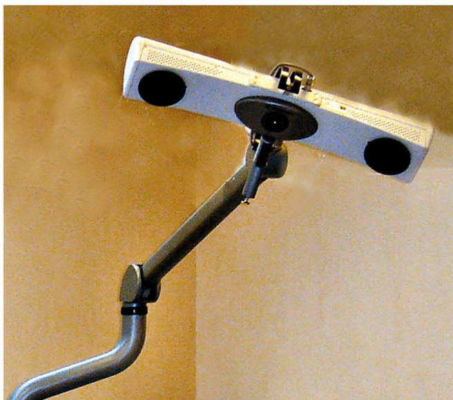
Figure 55.7 An infrared optical tracking system. In the centre of the gantry is a laser light that is used to position the arm during the set-up procedure.
